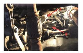
Remove the original injectors (see the 3 other page if necessary)
